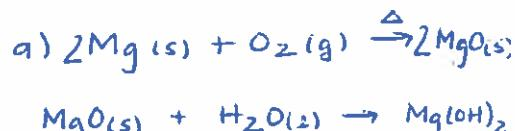
Magnesium is burnt in oxygen to produce X. X is then reacted with water.
